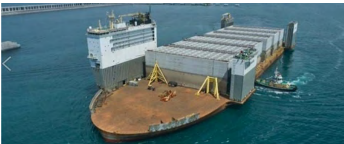
Diagram 3-5: Image of a previous caisson loading operation onto semisubmersible vessel at Langosteira Port.
