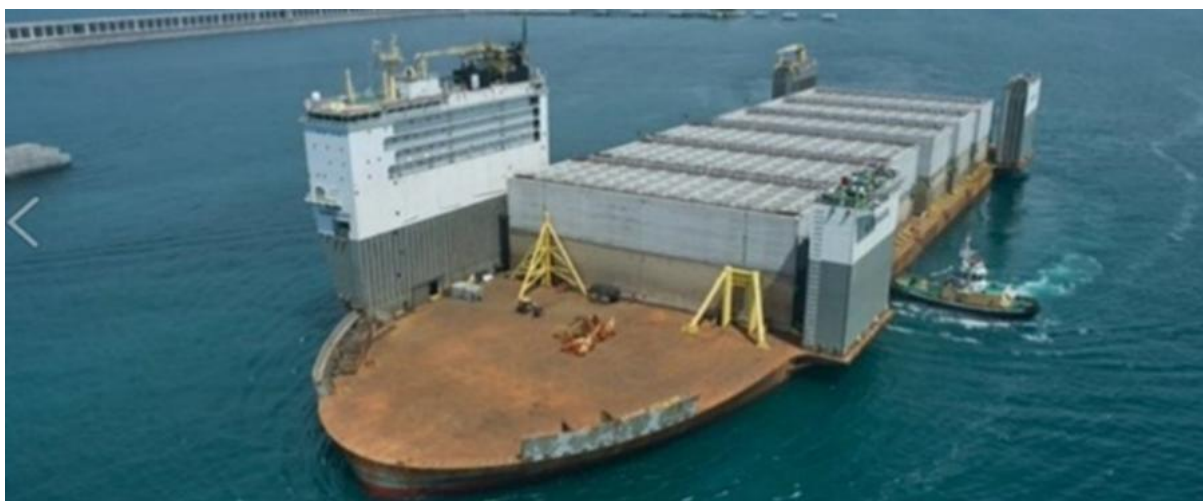
Diagram 2-6: Image of a previous caisson loading operation onto semisubmersible vessel at Langosteira Port.
