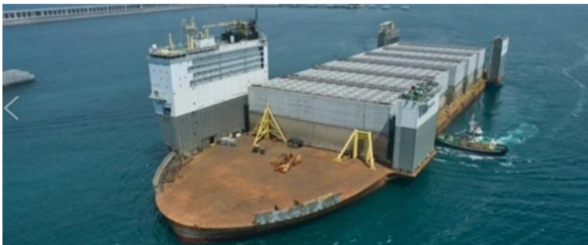
Diagram 2-6: Image of a previous caisson loading operation onto semisubmersible vessel at Langosteira Port.
